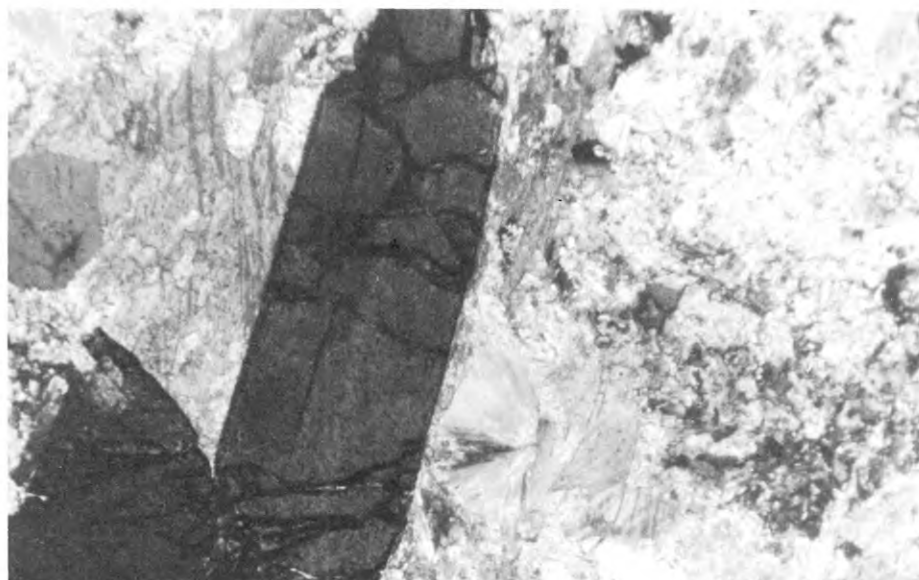
Fig. 10. Photomicrograph of a cassiterite crystal appearing as an elongated tetragonal prism (crossed polars)
