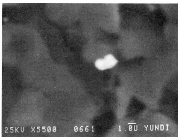
Fig. 8. Cassiterite (white) in tourmaline-bearing gravel from basal conglomerate of the Banxian Group in Xiangfen, Rongshui, Lowcheng
