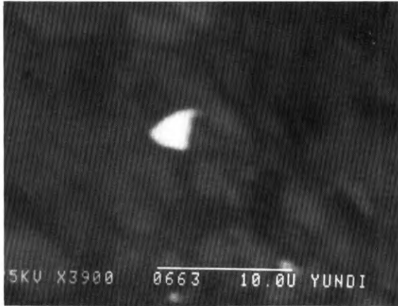
Fig. 5. Cassiterite inclusion in actinolite from Cu-Ni ore in the Baotan of Huonggang, Low-cheng
