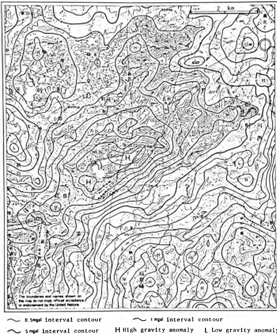
Figure IX. Gravity survey, Hishikari mine area ( D = 2.4 \text{ g/cm}^3 ). The contour lines show generally an ENE-WSW elongation, which is that of Au veins, but a NW-SE direction is seen in the northwestern part. The Hishikari deposit is located in the higher anomaly zone over 13 mgal. Yamada satellite deposit is situated at the southern part. Refer Figures VI and VII for the better vein location.
