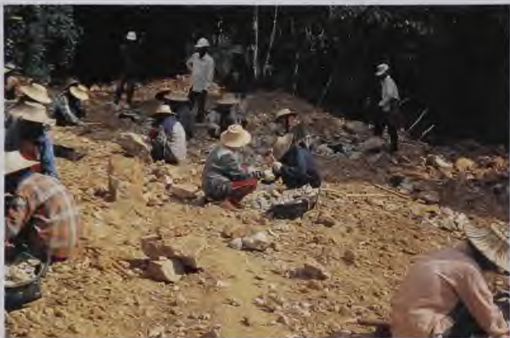
Hand-sorting ceramic-grade feldspar from pegmatite, Thailand. Photograph courtesy of Mr. D.E. Highley, British Geological Survey.
