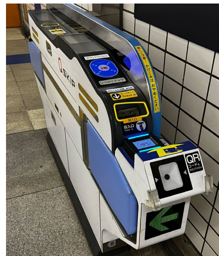
FIGURE 8.5 Ticket reader in a Japanese metro station for IC card, ordinary paper ticket, smartphone ticket, and QR code ticket
