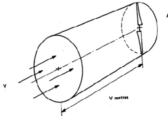
Wind power equipment extracts the kinetic energy in the wind and this form of energy cannot be stored like water at a higher elevation. These devices work more like 'run of the river' convertors. There are two distinct ways this is done. One depends on the drag effect where the rotor runs in the same direction as the wind itself. The other method utilizes the aerodynamic effects of the air passing over the airfoil shapes.
