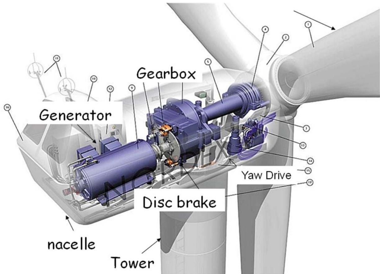
Figure 1.8 A typical modern Wind turbine
