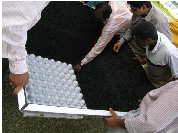
SODAR being set up for measurements
