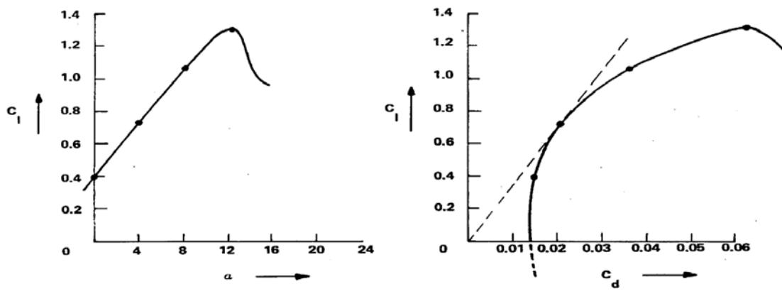
Figure 1.4 Dependence of Lift and drag coefficients on angle of attack (adopted from H.Lyson 1979)
