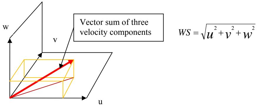
Figure 2.3 Three components of wind speed.
