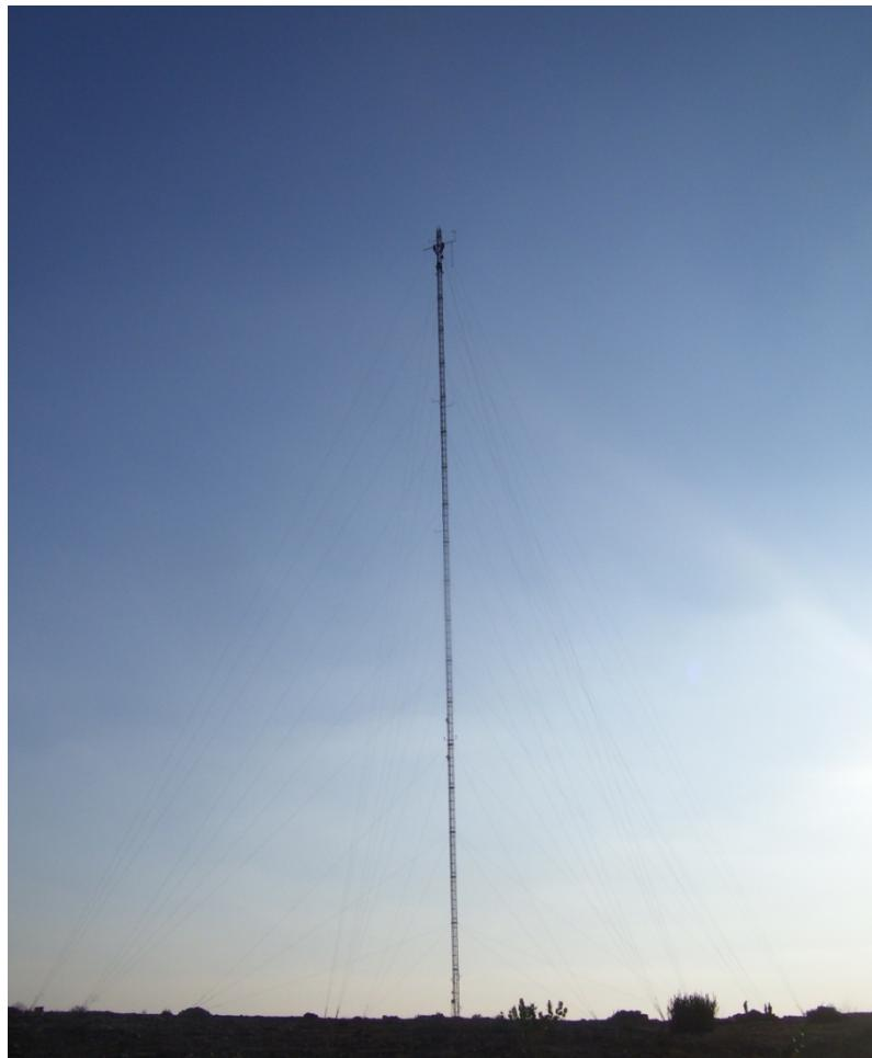
Figure 2.2 A typical wind monitoring mast.
