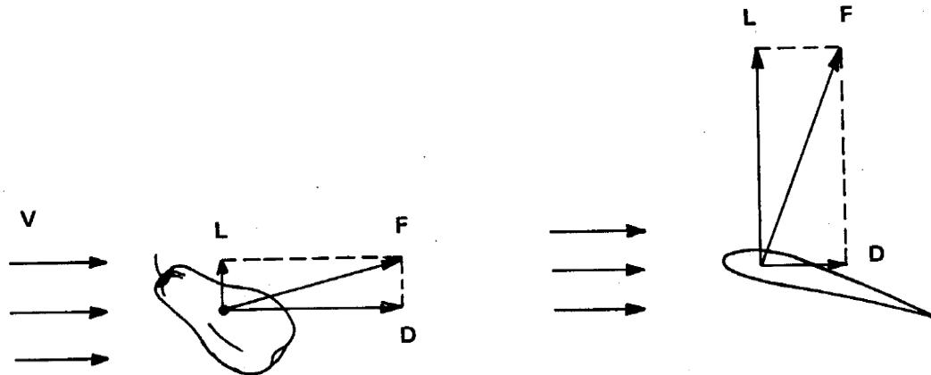
Figure 1.4 Lift and drag forces on a body immersed in fluid flow (adopted from H.Lyson 1979)
