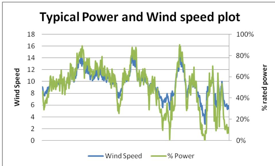
Figure 3.1 Typical time series plot of wind speeds and corresponding power
