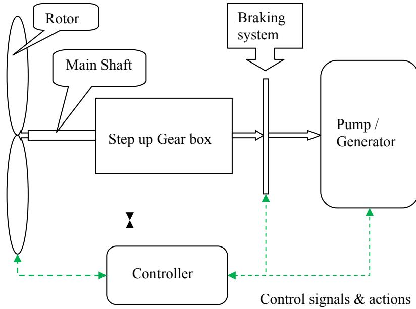
Figure 1.7 Components of a typical Wind Energy Convertor
