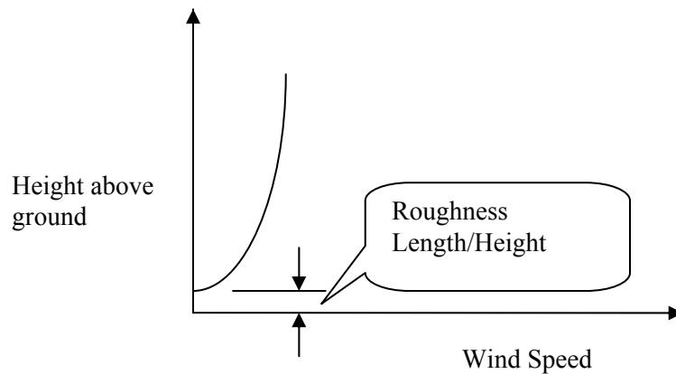
Most commonly used method for determining wind speeds at a height above ground referred to as the power law index method.
