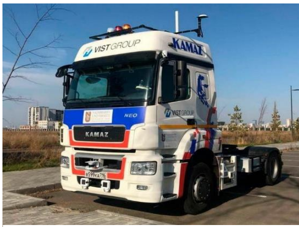
Figure 12. Driverless truck built on the basis of KAMAZ-5490 Neo.
