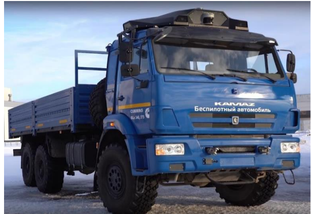
Figure 23. KAMAZ-43118 flatback truck equipped with “Avatar” kit.
