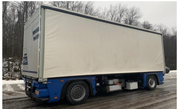
Figure 25. Prototype of cabinless freight vehicle by NAMI on a test run.
