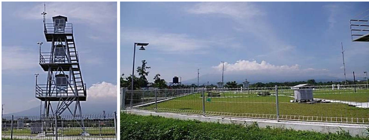
Figure 5.2 Towering Climatology, a tower to put microclimate measurement devices at various above ground altitude (left). A hut to protect the outdoor climatology measurement devices (right)
