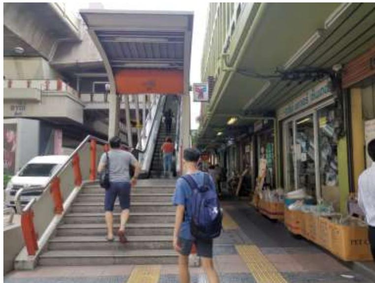
**Figure 5-2 Metro Station Stairways Taking more than Half of Walkway Width**
